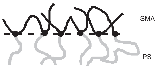
Fig. 50. Possible mechanism by which chains with multiple reactive sites can graft to an interface. This example, which would be typical of a maleic anhydride functionalized polymer reacting on a polyamide, shows on one side end-grafted chains and on the other side of the interface, a loop structure. The effect of this loop structure on the mechanical strength of the interface is not fully clear but loops that are too short will weaken the interface
